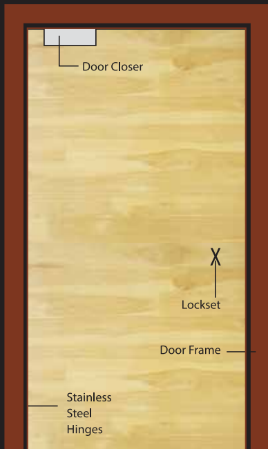
Door Frame Size - Single Leaf (maximum size 1220mm x 2440mm)
