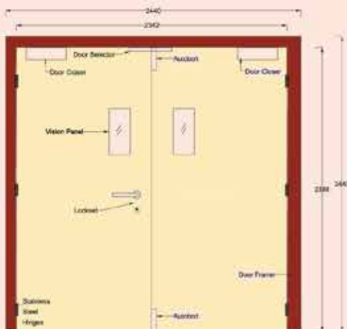
Door Frame Size - Two Hour Double Leaf (maximum size 2440mm x 2440mm)
