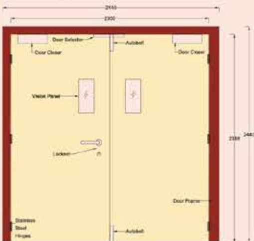
Door Frame Size - One Hour Double Leaf (maximum size 2440mm x 2440mm)
